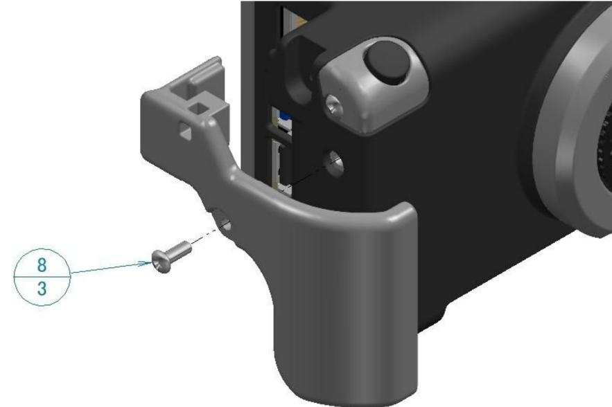
The shape of the clip is just one example. By using the spacers embedded in the clip, it is possible to attach accessories freely.
